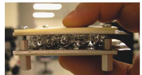
Shell array to increase detection efficiency.
